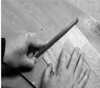
Proper position for squaring up an edge or smoothing a rough spot
