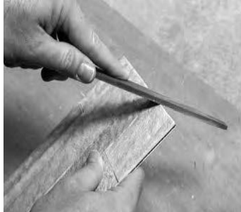
Do not file the edge at an angle
